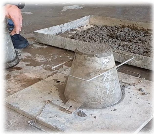
Figure 1: Slump test.
