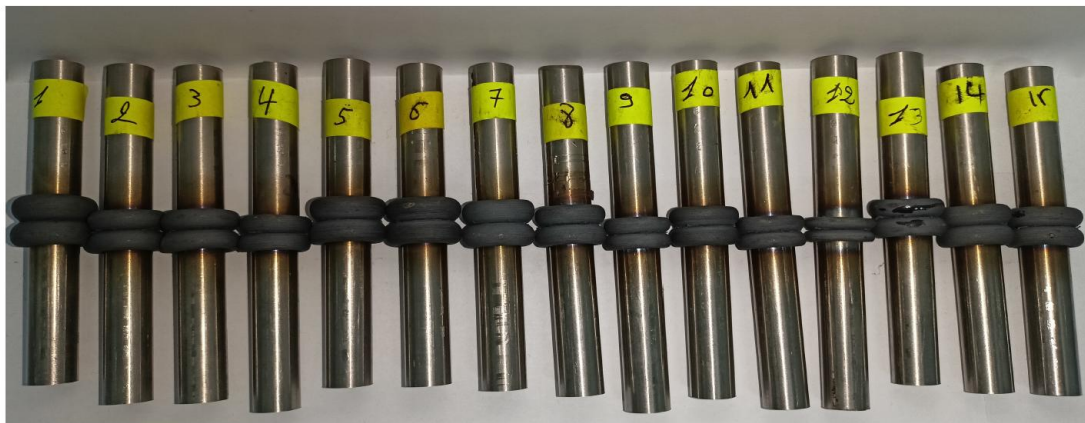
Figure 1. Welded test pieces
